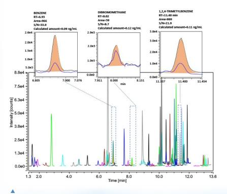
SIM trace showing the target compounds in a tap water sample spiked with a VOC mix at the lowest calibration point (0.1 ng/mL). Calculated MDL is  $\leq$ 0.17 ng/mL for all the compounds (MDL for BTEX is 0.01 ng/mL).
